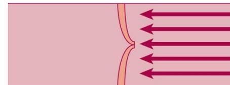
Valve closed; does not open in opposite direction
